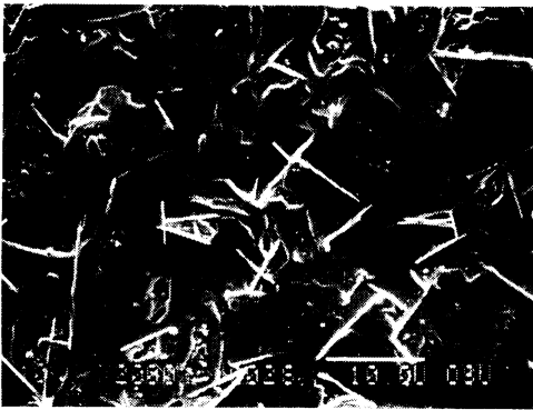
Fig.12 SEM photographs of the free surface of sample I under the annealing conditions of (a) 850^{\circ}\text{C} \times 8\text{ h} (non-superconducting), (b) 850^{\circ}\text{C} \times 5\text{ h} (superconducting), (c) 830^{\circ}\text{C} \times 5\text{ h} (non-superconducting).
